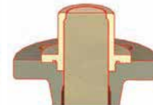
Model 28KS Metal seal in the vessel
