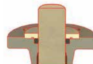
Model 28KV Radial soft seal in the valve body
