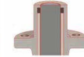
Model 26FR Extended body with a radial seal
